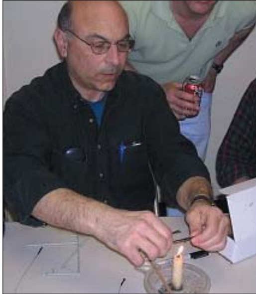
Bob demonstrates heating the technique for evenly heating a length of sprue over a candle flame prior to stretching it to create a fine thread. (PHOTO BY BOB DOEBLEY)
