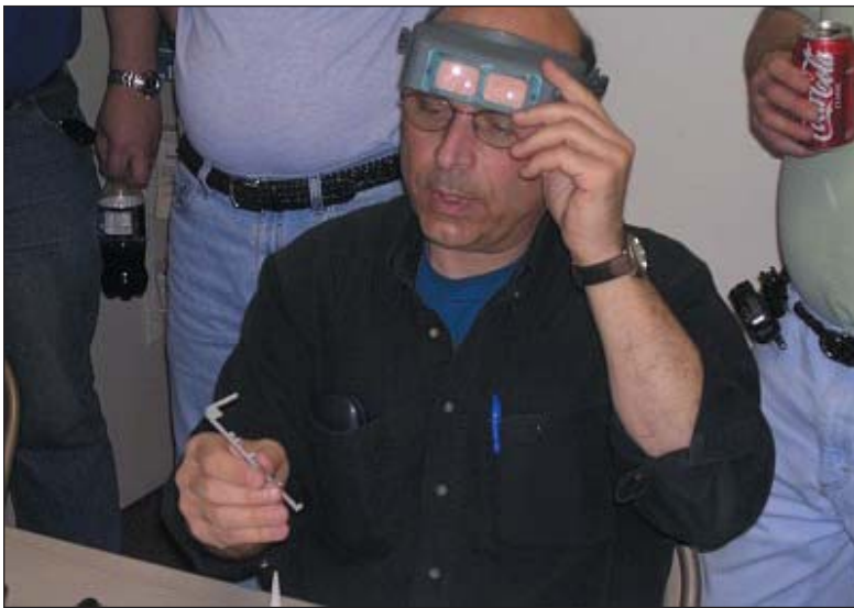
Bob used a bit of parts tree to demonstrate his rigging technique. Here he waits for a length of monofilament cemented in place to setup before tightening with heat from a lit incense stick.
